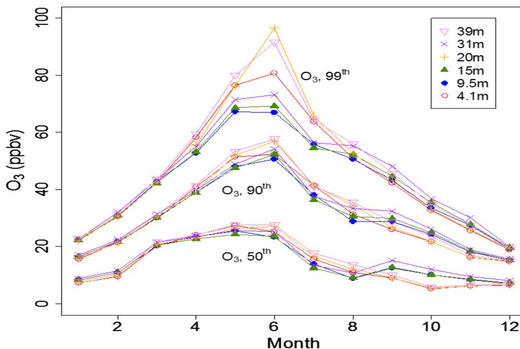
Figure 4. Monthly distributions of the 50th, 90th, and 99th percentiles of O<sub>3</sub> concentrations at six heights measure during 2011~2014.
