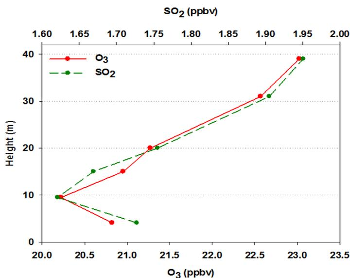
Figure 6. Average vertical profiles of the O<sub>3</sub> and SO<sub>2</sub> concentrations measured during 2012~2013.
