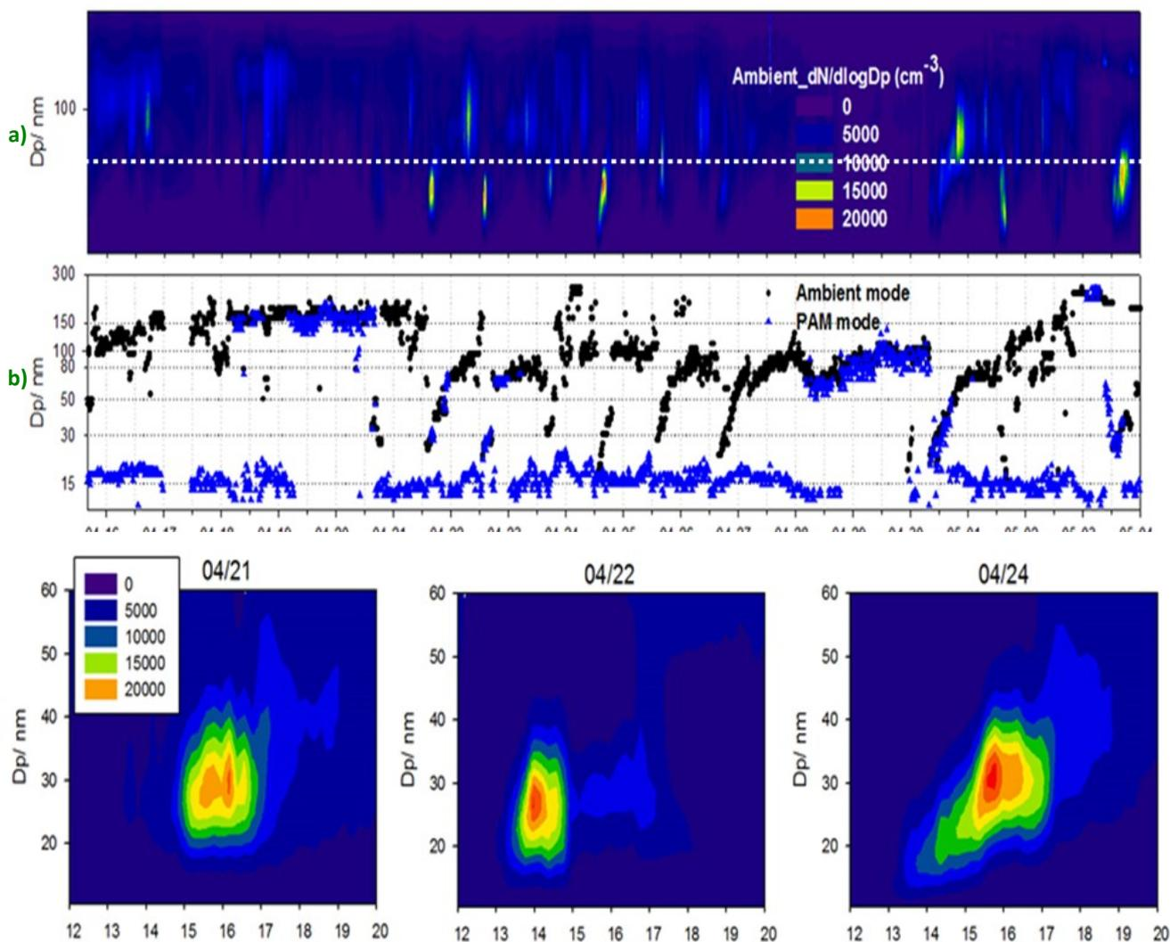
Figure 8. Size resolved number of aerosols between 10~500 nm measured at TRF during April ~ May 2014. a) number concentrations, b) mode diameters, and number concentrations for several days when particle growth were observed on 21, 22, and 24 April.
