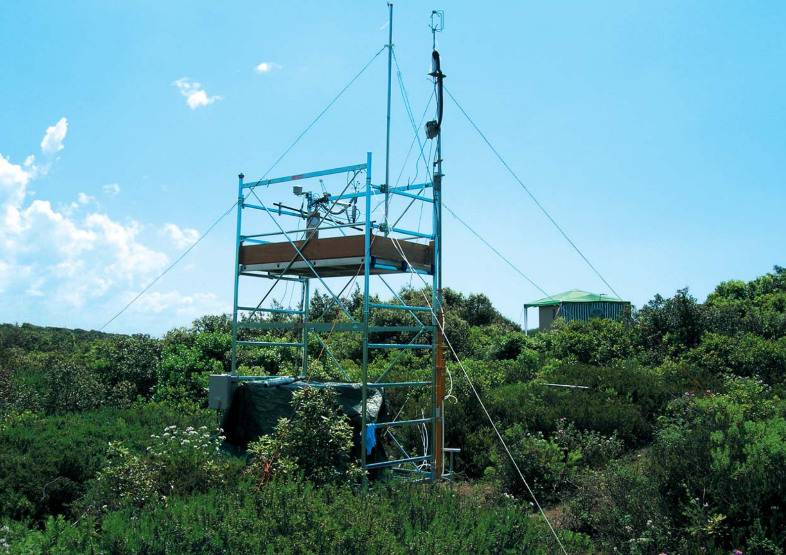
Figure 2. VOCBAS facilities for field measurement of VOC emission and reactivity: The equipment for VOC flux measurements by micrometeorological techniques (disjunct eddy covariance) during the ACCENT–VOCBAS campaign in Castelporziano (Italy).
