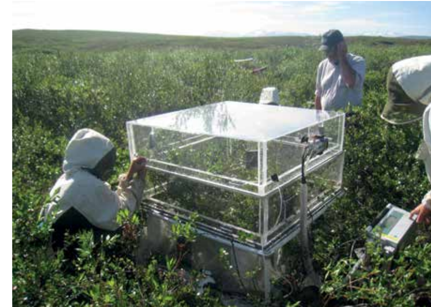
Figure 3. Measuring gas exchange from an Alaskan Arctic shrub canopy using a chamber and infra-red gas analyser, near Toolik Lake, Alaska. Short stature canopies allow direct measurements of structure, gas exchange, leaf traits and soil states. The Arctic Long Term Ecological Research site at Toolik Lake has pioneered studies on tundra responses to global change.
