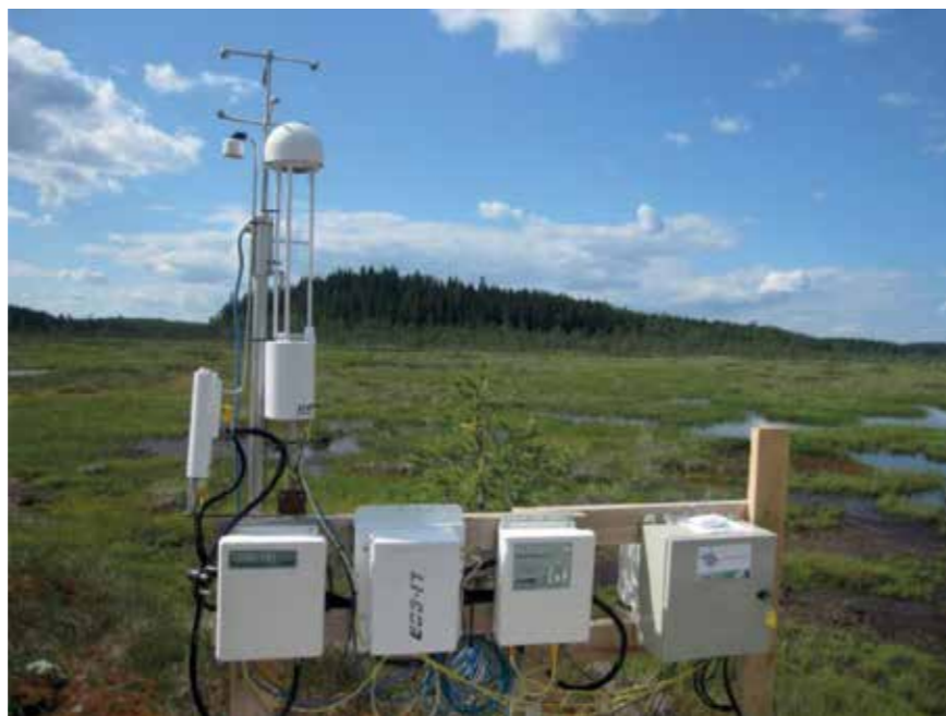
Figure 2. Eddy covariance measurement set-up for methane and carbon dioxide at Siikaneva bog wetland in Finland (Photo: Timo Vesala)
