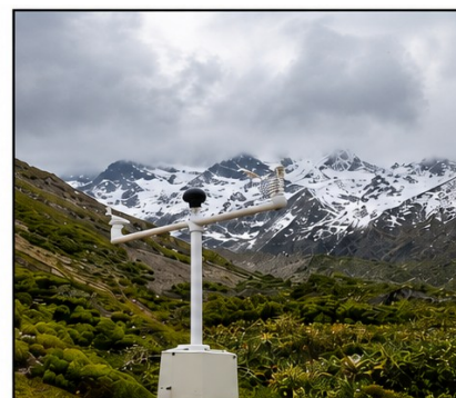
(c) Automatic Weather Station recording meteorological parameters
